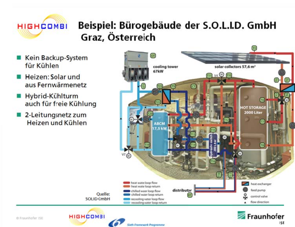
One of the presentation slides (High Combi System at S.O.L.I.D., Graz, Austria)
